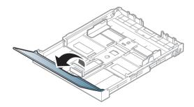
Press and unlatch the guide lock in the tray, pull the tray out manually. Then adjust the paper length guide and paper width guide.
